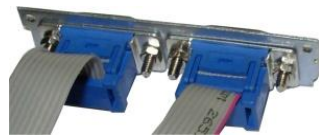
Two DB9 connectors mounted on a back plate
