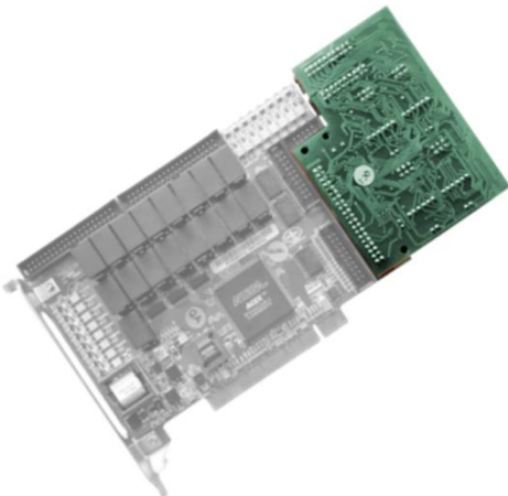
The PSP-1400-D is “piggyback” mounted to the PIO-1000 I/O module
